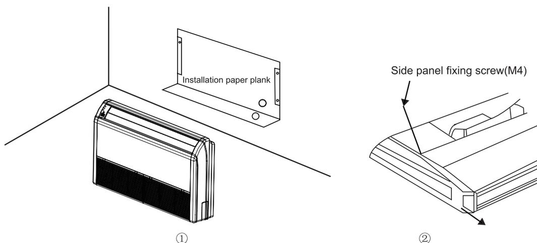
(2) Remove the return grill, the side panel and the hanger bracket from the indoor unit as per procedure below.
