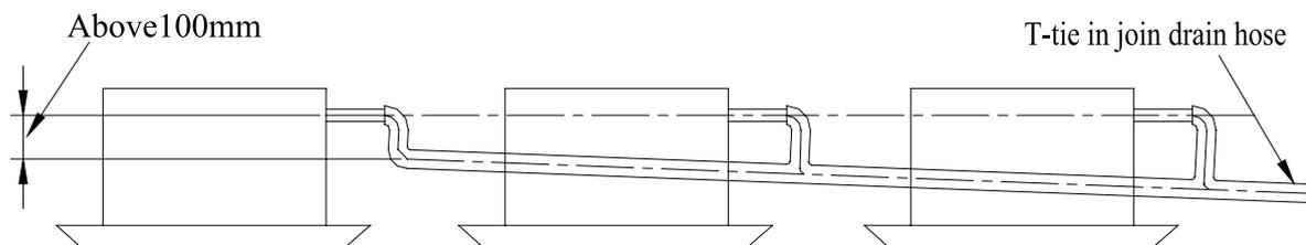
The specs of the selected join drain hose should fits the running capacity of the unit.
