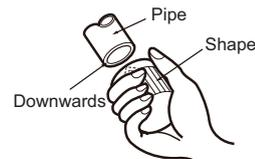
C: Put on suitable insulating pipe
