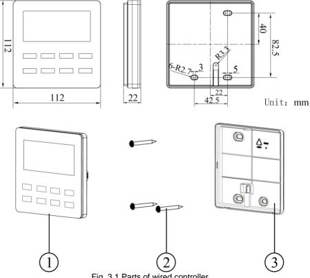
Fig. 3.1 Parts of wired controller
