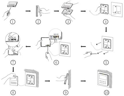
Fig. 3.7 Installation diagram for wired controller
