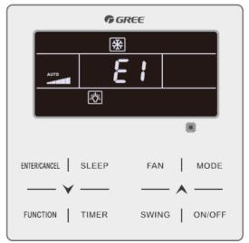
Fig.5.1 Display of Outdoor Unit High Pressure Protection
