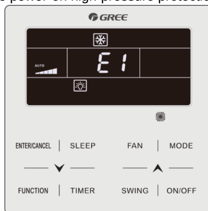
Power-on High-pressure Protection Fault Interface
