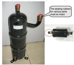
**Note:** Compressor lubricant must be kept completely airtight. Hitachi compressors use special lubricant FVC68D whose moisture absorption capability is high. Requirements on air-tightness of these compressors are higher.
