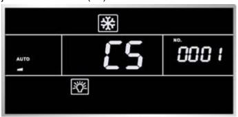
If this fault occurs, the number of the new AP1 is identical to that of a unit within the network. Manually change it to the original number of the faulty AP1 or a unique number. There are three methods to change project number:
