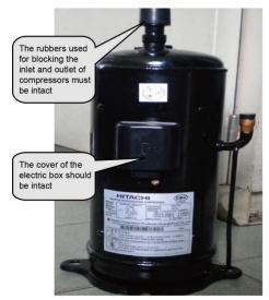
*Note:* The new compressor must be consistent with the faulty one in model.
