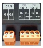
CAN Interface: It is connected to the air conditioning system through twisted pairs so as to get through the communication between the Modbus gateway and the air conditioning system.
