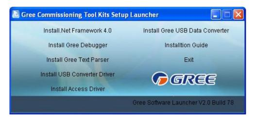
If it is the first time to use Gree Debugger, the following software needs to be installed: .Net Framework 4.0, USB Converter Driver, Access Driver (required for versions earlier than Office 2007), and Gree Debugger.
