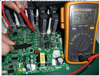
6) As shown in the figure below, put the black test probe to pad V (YE) and the red test probe to pad NV (make sure the moisture proof tape is removed). In normal cases, the multimeter should read 0.39±0.3 V. If it is "0" or infinitely great, the IPM module is faulty.
