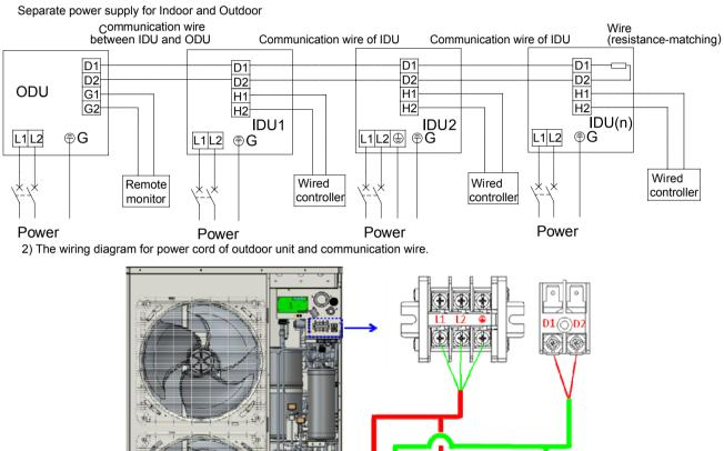
There are two wiring diagrams for communication wires of indoor/outdoor units and remote monitor:
