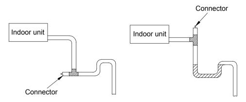
8.1.5 During condensate water pipe installation, ensure a distance above 500 mm between the pipe and the electric box of the unit for maintenance. In a case when the space is not enough, the final piping way must be determined by the technical personnel.
