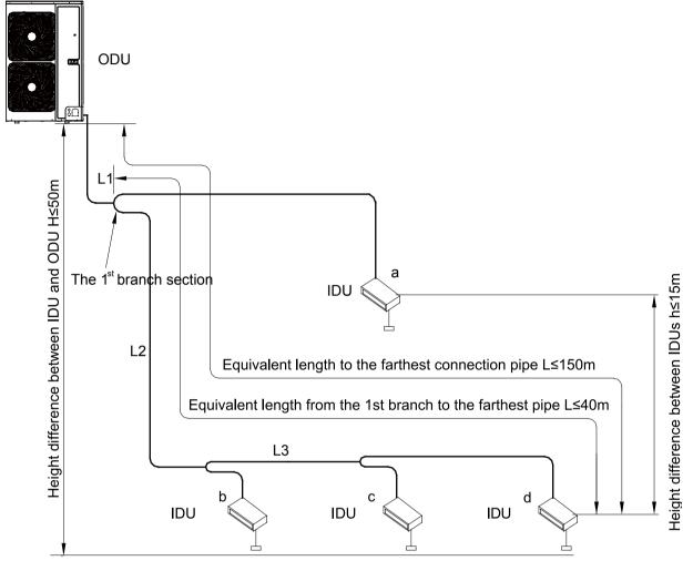
Each Y-type branch equals to 0.5m and each branch header equals to 1.0m.
