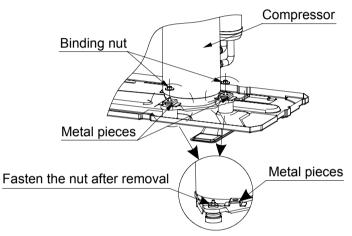
When installing the unit, metal pieces for transportation must be removed. Then fasten the binding nuts again and wrap back soundproofing cotton.
