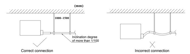
When connecting the drain pipe to that of the IDU, fix the pipes with the bands provided upon delivery instead of using the glue to facilitate further maintenance.
