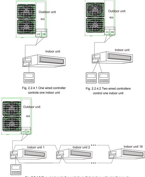
Fig. 2.2.4.3 One wired controller controls multiple indoor units simultaneously
