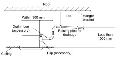
c. The drain pump shall be fixed securely. Otherwise, abnormal noises will be generated.
