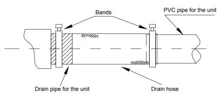
e. Apply insulation materials to the condensate water pipe joints to prevent dewing. d. Insulation for connection between the drain pipe and that of the IDU is shown in the following figure.
