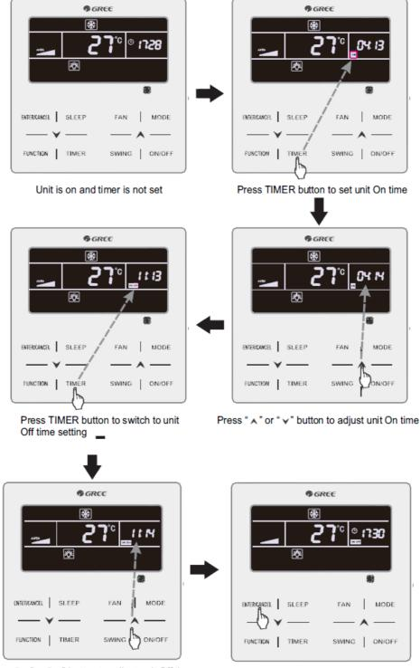
ess " ^ " or " v " button to adjust unit Off time
