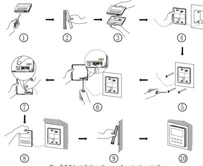
Fig. 2.2.2 Installation diagram for wired controller
