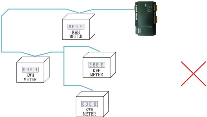
The number of KWH meters connected to one gateway should not exceed 15.
