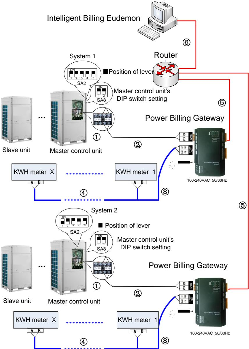
(1) Communication cable connection between gateway and air conditioners:
