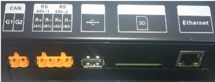
**CAN communication port:** Connect to air conditioners via two-core communication cable to obtain data from air conditioners;
