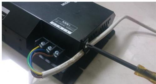
Note: Power cord should be fixed with the wire clip in the toolkit, as shown in the picture.
