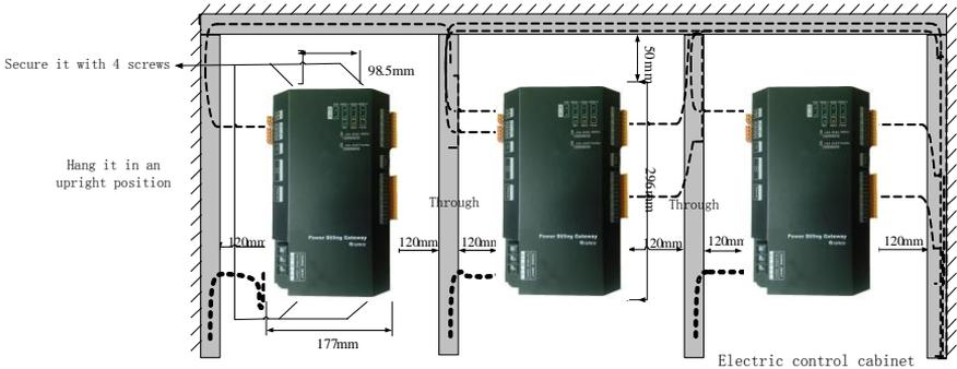
Power cord and communication cable of the gateway must be arranged separately; otherwise malfunction will occur to the gateway!
