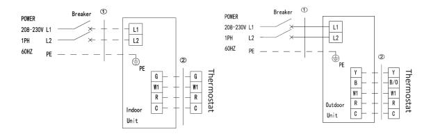
Note that the indoor unit features an onboard 24VAC transformer, rated at 40VA.
